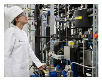
High-pressure super critical fluid extraction (SFE) pilot plant
