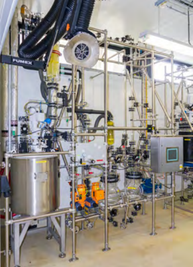
Left: 100-liter reaction and distillation unit
