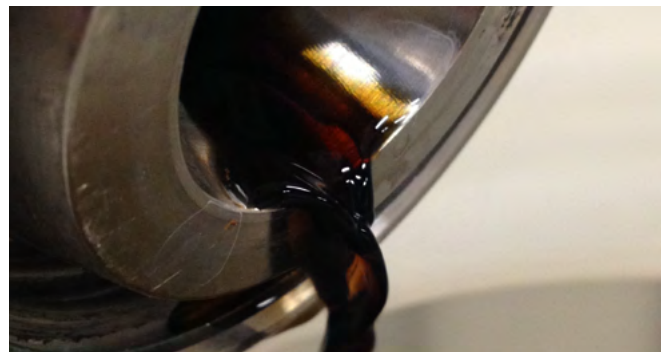
Lignin cleavage solution from the high-pressure plant
