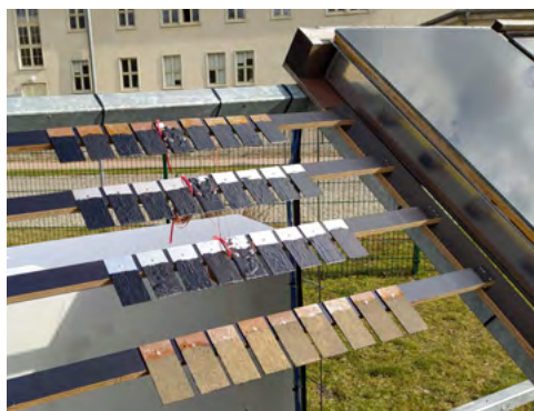
left: Coatings made from lignin-based bitumen
