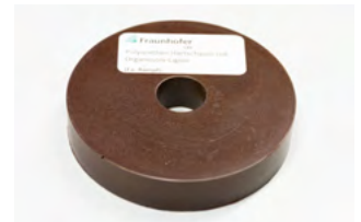
Polyurethane rigid foam with Organosolv lignin
