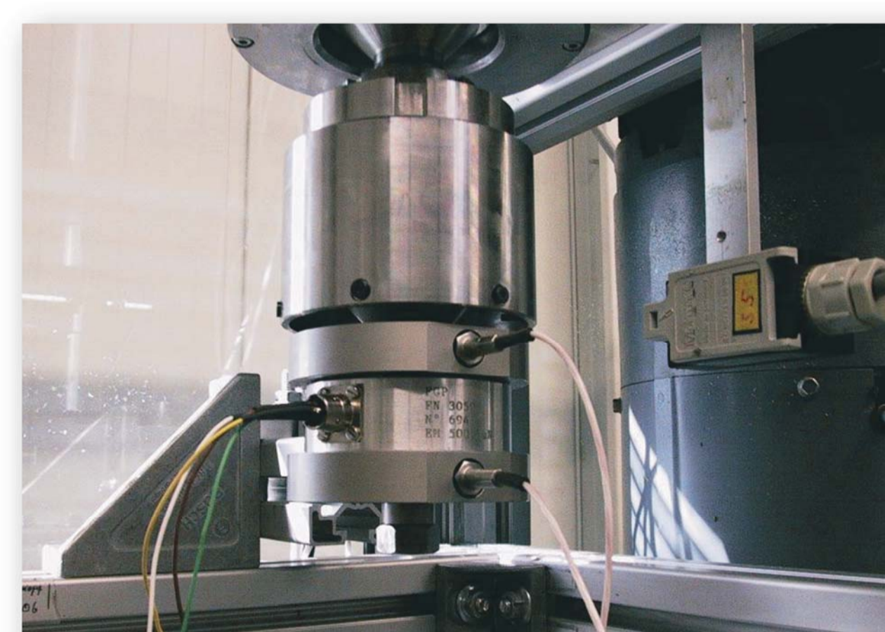
Figure 9: Test rig for friction measurement test bearing 6001/7001
